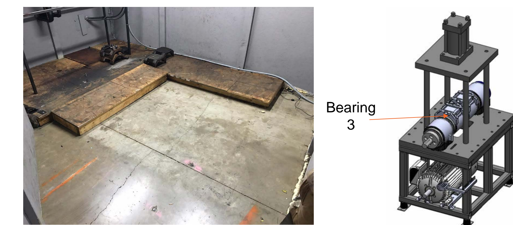
Figure 1: (Left) The test rig will be constructed and operate in this 90" x 132" x 90" room. (Right) CAD model of the new four bearing test rig.
